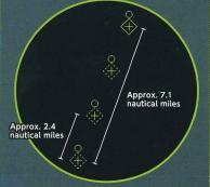
For vessels equipped with AIS, only the symbol marks\* appear on the radar screen. The center line is not displayed.
